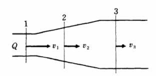
To get flow velocities v<sub>1</sub>, v<sub>2</sub> and v<sub>3</sub>
