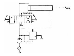
The speed of extension is greater than that for a regular double-acting cylinder because flow from the rod end (QR) regenerates with the pump flow (Qp) to provide a total flow rate (Qr), which is greater than the pump flow rate to the blank end of the cylinder The operation of the cylinder during the retraction stroke is the same as that of a regular double-acting cylinder.
