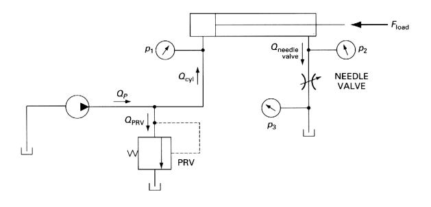
First we solve for the rod end pressure  $p_2$  that causes the blank end pressure  $p_1$  to equal the PRV setting. This is done by summing forces on the hydraulic cylinder.
