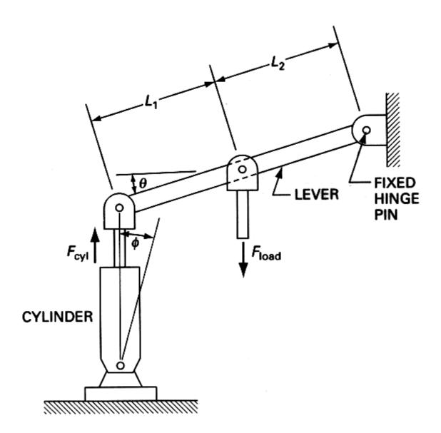
$$F_{\text{cyl}} \cos \phi \ (L_1 + L_2) \cos \theta = F_{\text{load}} (L_2 \cos \theta)$$
