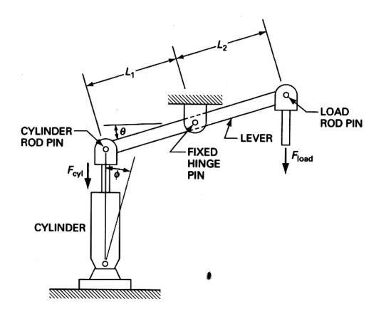
$F_{\text{cyl}}(L_1 \cos \theta \times \cos \phi) = F_{\text{load}}(L_2 \cos \theta)$  $F_{\text{cyl}} = \frac{L_2}{L_1 \cos \phi} F_{\text{load}}$
