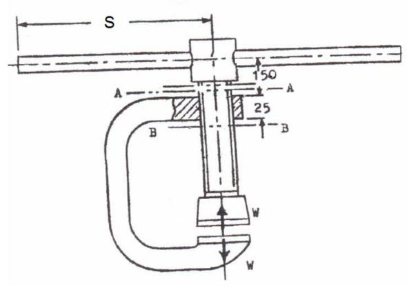
The 70 mm double thread screw of a 10 kN shop press, shown in Figure, has an iso-trapezoidal thread. The operator's force may be taken 180 N for each hand. The mean diameter of collar is 60 mm. Determine:
