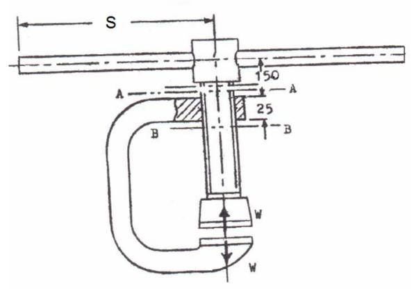
The 70 mm screw of a 10 kN shop press, shown in Figure, has a trapezoidal thread with an angle of 28. The operator's force may be taken 180 N for each hand. The mean diameter of collar is 60 mm. Determine:
