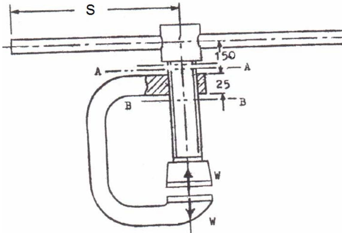
The 70 mm screw of a 10 kN shop press, shown in Figure, has a square thread. The operator's force may be taken 180 N for each hand but he is using only one hand. The mean diameter of collar is 60 mm.
