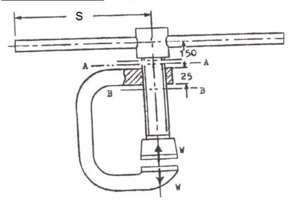
The 70 mm screw of a 10 kN shop press, shown in Figure, has a square thread. The operator's force may be taken 180 N for each hand but he is using only one hand. The mean diameter of collar is 60 mm.
