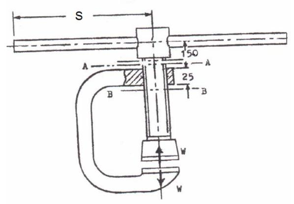
The 70 mm screw of a 10 kN shop press, shown in Figure, has a square thread. The operator's force may be taken 180 N for each hand but he is using only one hand. The mean diameter of collar is 60 mm. Determine:
