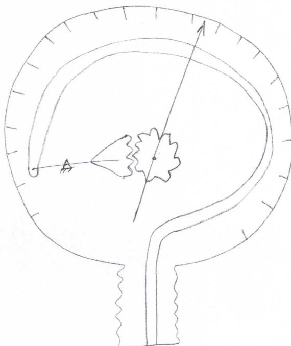
\* For measuring pressure in almost all ranges except minutely small press
