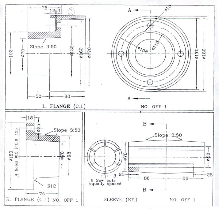
You are given the details of <u>COMPRESSION COUPLING</u>. Assemble all parts using 4 M10 through bolts. Draw the following views:
