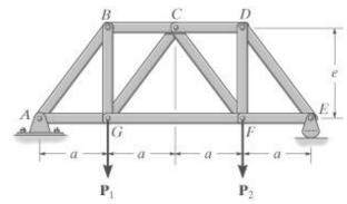
4- In the frame shown, determine the vertical and horizontal components reactions at pins B and C.
