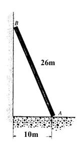
5- The uniform pole has a weight of 30N and a length of 26m. If the it is placed against the smooth wall and on the rough floor in the position shown in figure. Will it remain in this position when it is released? The coefficient of static friction  $\mu_s = 0.3$ .
