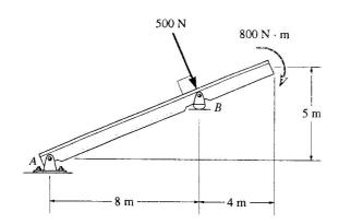
2- Determine the magnitude of the reactions on the beam at A and B. Neglect the thickness of the beam.
