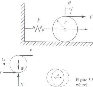
**Figure 3.26** Free-body diagram of wheel.
