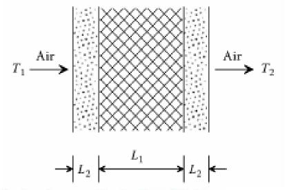
a. The heat transfer through the insulated wall can be represented using a thermal circuit with five thermal resistances connected in series as shown in Figure 7.30. Two modes of heat transfer, conduction and convection, are involved. The corresponding thermal resistances are
