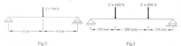
3) For the beams shown in figure 4 calculate the maximum bending stress
