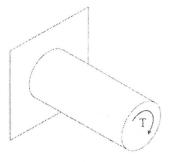
7) For the shown machine member 5 cm diameter. Find the maximum normal stress in the member and its point of action.
