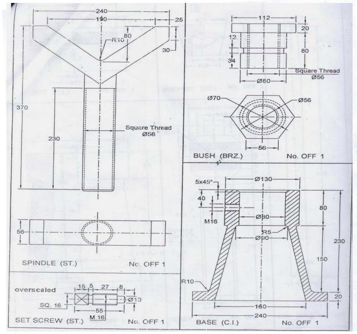
You are given the details of a <u>SCREW JACK</u>. Assemble all parts and draw the following views: a) SEC. ELEVATION
