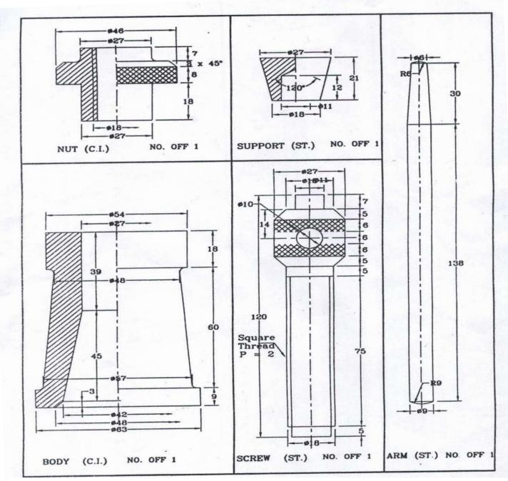
You are given the details of a **SCREW JACK**. Assemble all parts and draw the following views:
