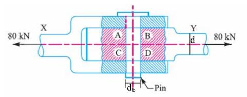
**Solution.** Given :  $P = 80 \text{ kN} = 80 \times 10^3 \text{ N};$  $\sigma_t = 100 \text{ N/mm}^2; \tau = 80 \text{ N/mm}^2$
