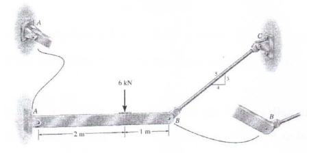
$$\frac{\text{pin } A}{F_A} = \sqrt{5.33^2 + 2^2} = 5.68 \text{ KN}$$
