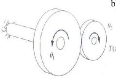
b) A shaft is fixed at one end and has the larger gear of a pair of gears at the other end. The pitch radii of the steel gears are r<sub>1</sub> = 8 inches (64 teeth) and r<sub>2</sub> = 4 inches (32 teeth); the tooth face widths are *T(t)* 0.5 inch. Find the equation of motion of this system if the smaller gear has a torque Tsinωt applied to it, where ω is the frequency, in rad/s, of the excitation torque.
