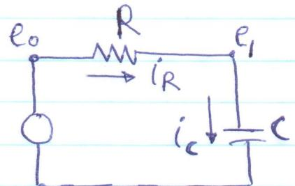
The circuit shown in figure has a resistance  $8\Omega$ , find the capacitance necessary to give a settling time  $2.5 \text{ mSec}$ .
