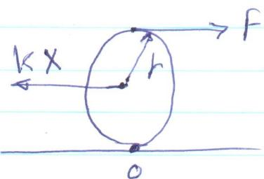
$$\begin{aligned}\sum M_O &= m\ddot{x}(r) + J\ddot{\theta} \\ \text{(+)} &= mr^2\ddot{\theta} + J\ddot{\theta} \\ &= [mr^2 + J]\ddot{\theta}\end{aligned}$$
