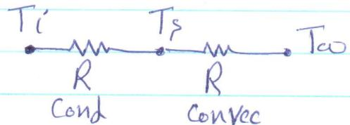
$$R_{\text{Cond}} = \frac{L}{kA} = \frac{0.006}{0.195 \times 0.1 \times 0.1} = 3.08 \text{ K/W}$$
