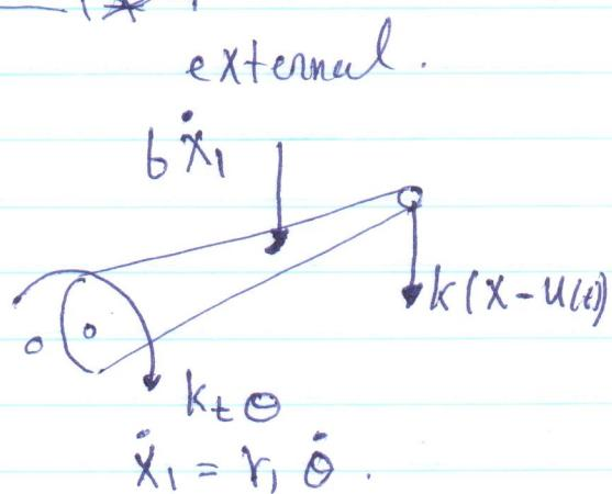
$$\begin{aligned} \sum M_o &= -k_t\theta - b\dot{x}_1(r_1) \\ (+) \uparrow \text{ext} & -kr_2(x - u(t)). \\ &= -k_t\theta - br_1^2\dot{\theta} - kr_2^2\dot{\theta} + kr_2u(t). \end{aligned}$$
