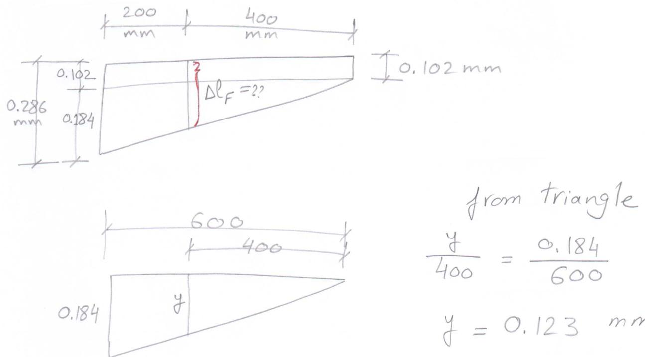
$$\begin{aligned}\Delta l_F &= 0.102 + y \\ &= 0.102 + 0.123 \\ &= 0.225 \text{ mm}\end{aligned}$$
