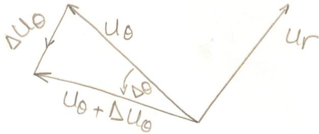
$$\begin{aligned}\vec{a} &= (r'' - r \dot{\theta}^2) \vec{u}_r + (2r' \dot{\theta} + r \dot{\theta}'') \vec{u}_\theta \\ &= a_r \vec{u}_r + a_\theta \vec{u}_\theta\end{aligned}$$
