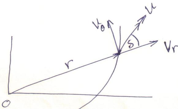
$$\begin{aligned}\vec{a} &= \dot{\vec{v}} \\ &= r'' \vec{u}_r + r' \dot{\vec{u}}_r + r' \dot{\theta} \vec{u}_\theta + r \dot{\theta}' \vec{u}_\theta + r \dot{\theta} \dot{\vec{u}}_\theta \\ &= r'' \vec{u}_r + r' \dot{\theta} \vec{u}_\theta + r' \dot{\theta} \vec{u}_\theta + r \dot{\theta}' \vec{u}_\theta - r \dot{\theta}^2 \vec{u}_r\end{aligned}$$
