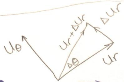
$$\left. \begin{aligned} \vec{v} &= \dot{r} \vec{U}_r + r \dot{\theta} \vec{U}_\theta \\ &= v_r \vec{U}_r + v_\theta \vec{U}_\theta \end{aligned} \right\} \begin{aligned} v &= \sqrt{v_r^2 + (v_\theta)^2} \\ \delta &= \tan^{-1} \frac{v_\theta}{v_r} \end{aligned}$$
