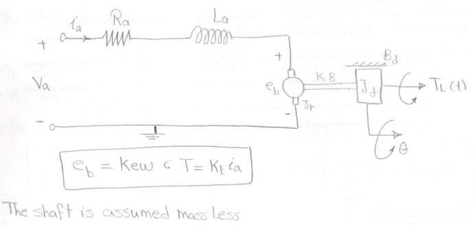
B = Coef. of torsional Viscous damping of the shaft K = brsional stiffness of the shaft Bj = Coef. of Viscous damp associated with the dish
