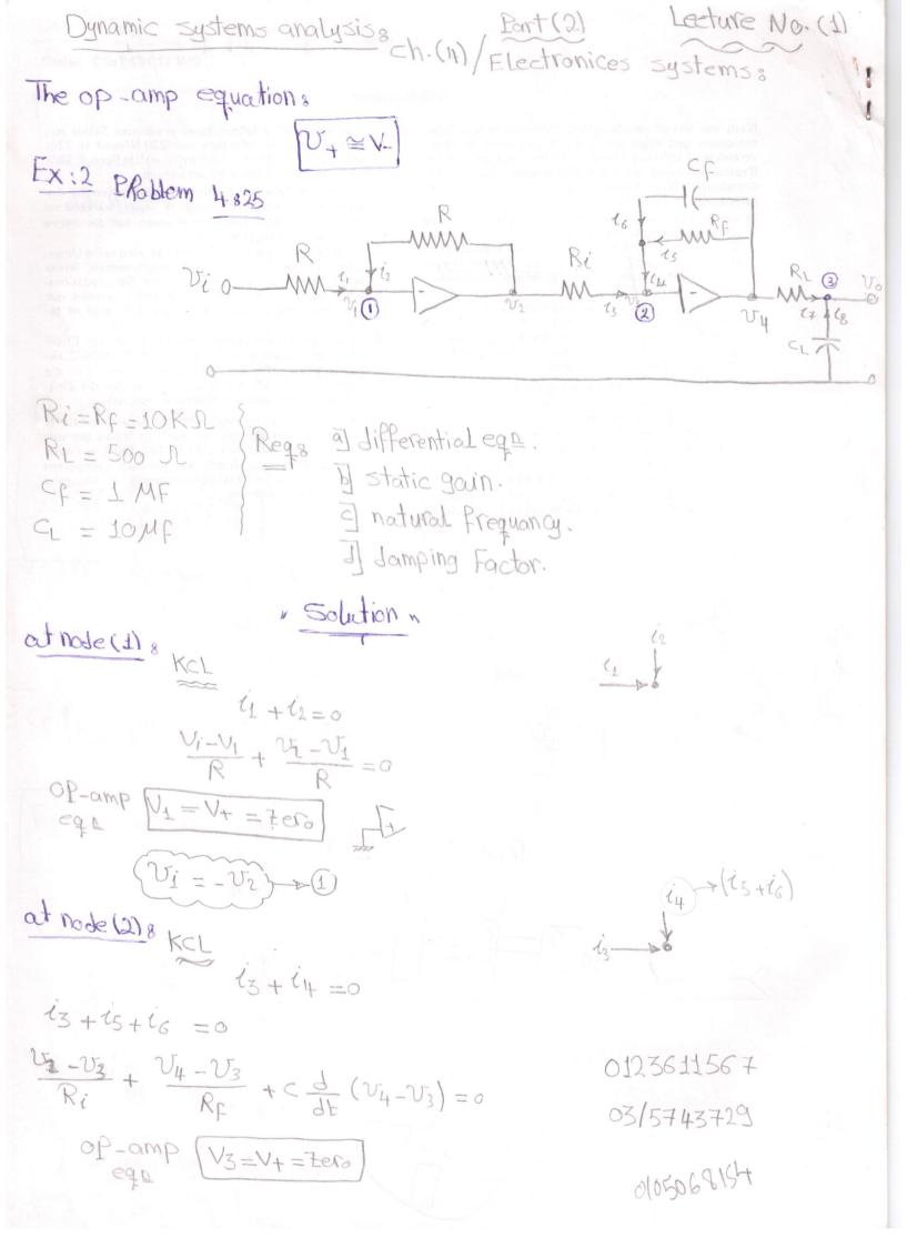
$$\frac{V_{2}}{R_{i}} + \frac{V_{1}}{R_{F}} + C_{F} U_{1}^{i} = 0 \longrightarrow 0$$
