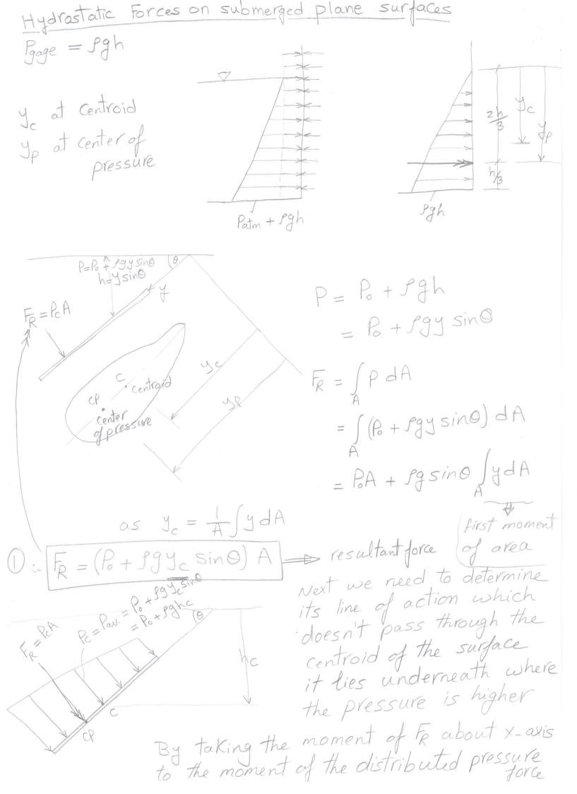
$$\begin{aligned} y_{p} F_{R} &= \int_{A} \frac{y}{p} P dA \\ &= \int_{A} \frac{y}{(B + p} gy \sin \theta) dA \\ &= E_{p} \int_{A} \frac{y}{dA} + fg \sin \theta \int_{A} \frac{y^{2}}{dA} \\ \hline y_{p} F_{R} &= F_{p} \frac{y}{dc} A + fg \sin \theta I_{xx,p} \end{aligned} \qquad (2) \end{aligned}$$
