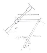
At a given instant the top end A of the bar has the velocity and acceleration shown. Determine the acceleration of the bottom B and the bar's angular acceleration at this instant.
