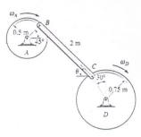
6 — Knowing that angular velocity of link AB is  $\omega_{AB} = 4 \text{ rad/s}$ , determine the velocity of the collar at C and the angular velocity of link CB at the instant shown. Link CB is horizontal at this instant.
