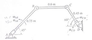
The flywheel rotates with an angular velocity  $\omega = 2 \text{ rad/s}$  and an angular acceleration  $\alpha = 6 \text{ rad/s}^2$ . Determine the angular acceleration of links AB and BC at this instant.
