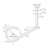
At a given instant the wheel is rotating with the angular velocity and angular acceleration shown. Determine the acceleration of block *B* at this instant.
