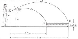
12-32  $\perp$  Determine the maximum height on the wall to which the firefighter can project water from the hose, if the speed of the water at the nozzle is  $v_C = 14$  m/s.
