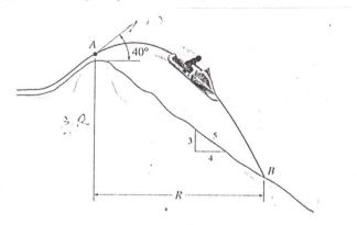
$12_{-10}$  A golf ball is struck with a velocity of 24 m/s as shown. Determine the speed at which it strikes the ground at B and the time of flight from A to B.
