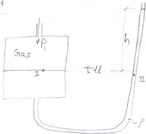
$$\begin{aligned} P_I &= P_{II} \\ P_1 &= \rho g l l + \rho g h \\ &= \rho g \times \frac{d^2}{D^2} h + \rho g h \\ &= \rho g h \left( \frac{d^2}{D^2} + 1 \right) \end{aligned}$$
