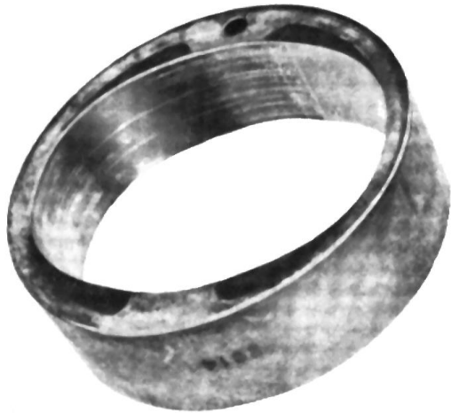
Rust caused by moisture in the oil
