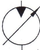
uni-directional variable displacement hydraulic Motor (ii)
